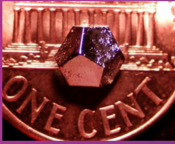
An optical micrograph of the perfect dodecahedral symmetry of the mm-sized, single icosahedral quasi-crystal \text{Ho}_{8.7}\text{Mg}_{34.6}\text{Zn}_{56.8} . Courtesy of I.R. Fisher
